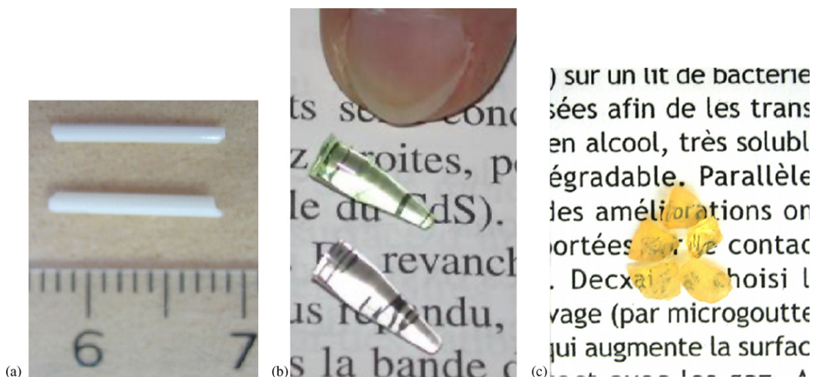
Fig. 1. Photos of (a) \text{TiO}_2 -QZ bars; (b) (top) a DCA-SG monolith; (bottom) a non-doped monolith; (c) ANT-SB beads.
